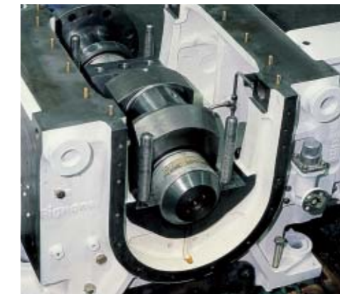
Main bearing split in the vertical plane.
