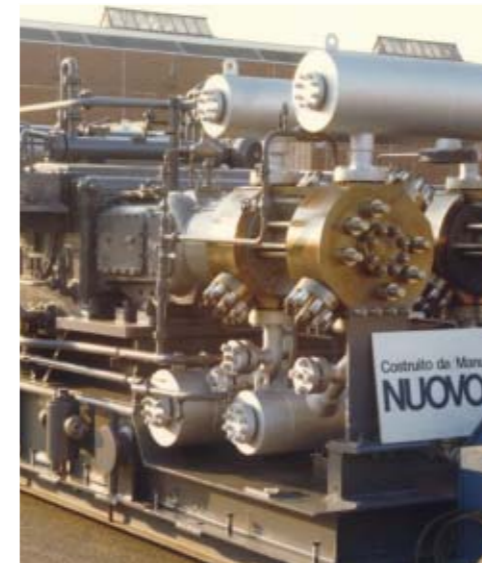
Re-injection compressor - model 4HE/2 at 370 bar.
