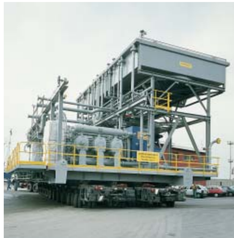
6HM reciprocating compressor offshore module during transportation.
