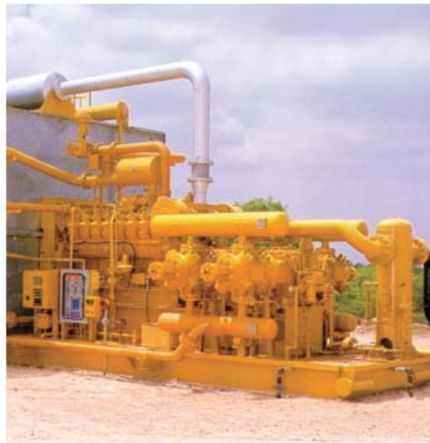
D6 API 11P gas engine driven packaged reciprocating compressor.
