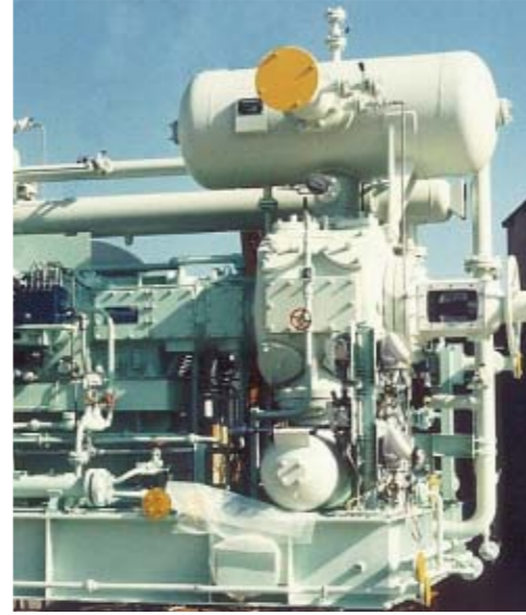
Polypropylene plant compressor package - model 2HA/2
