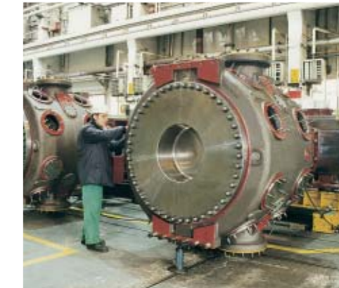
Large bore cylinder during assembly.
