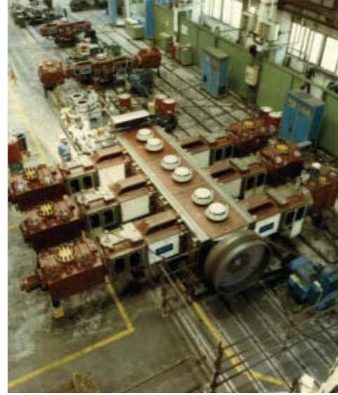
Hydrogen Make-up compressor - model 6HG/4 during shop test.
