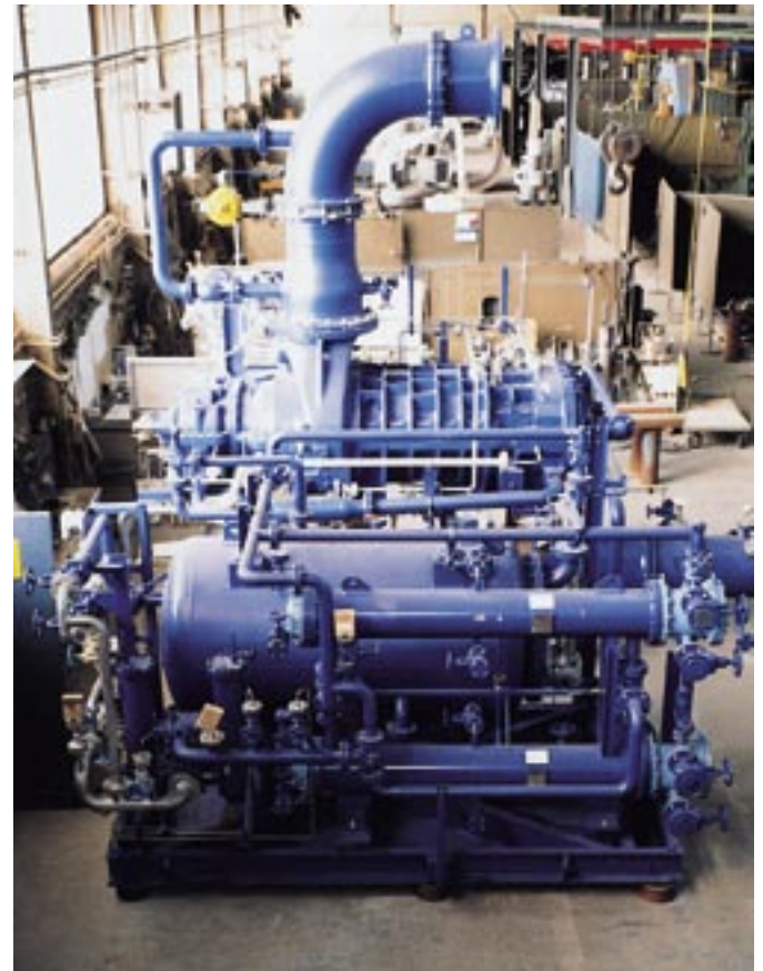
Kaucuk A.S., Kralupy (Czech Republic) Compression of styrene gas VRa 736 L – intake volume flow of 28.000 m 3 /h Compression of 0,28 to 1,62 bar (abs.) Sealing by carbon labyrinth rings with nitrogen as seal gas
