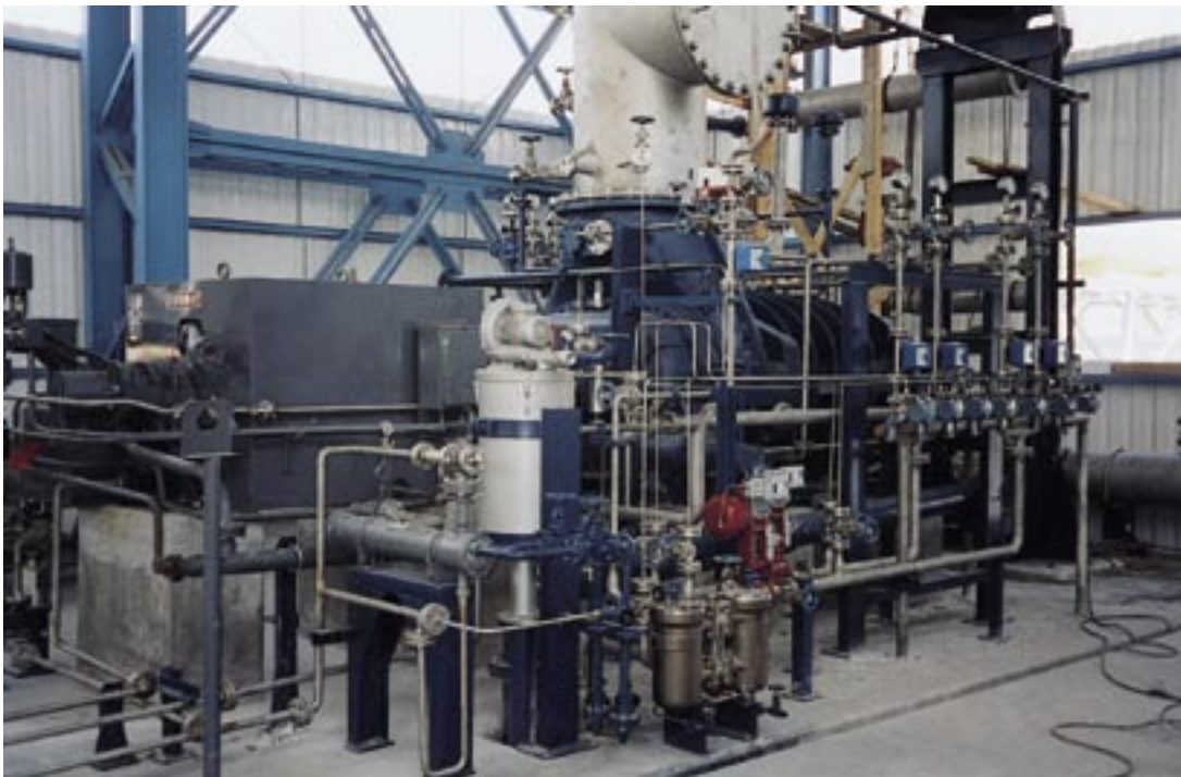
Soda Sanayii, Mersin (Turkey), compression of coke oven gas VRO 836 L, intake volume flow of 45.000 m 3 /h, compression of 0,85 to 3,5 bar (abs.), water-purged carbon labyrinth sealing
