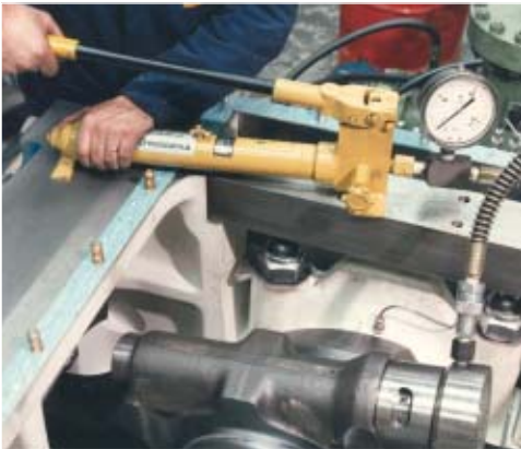
Connecting rod hydraulic tightening.
