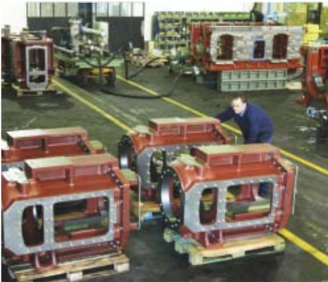
Crosshead extensions of HF frame.
