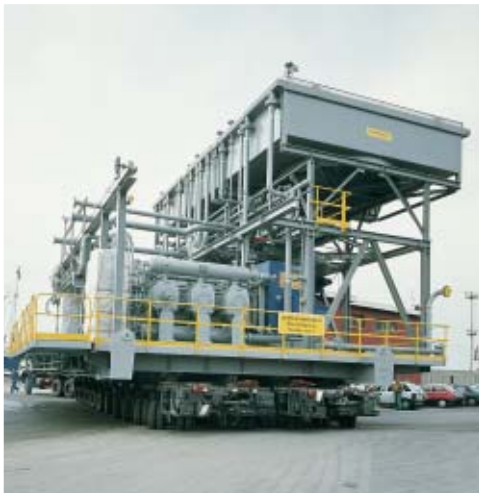
6HM reciprocating compressor offshore module during transportation.
