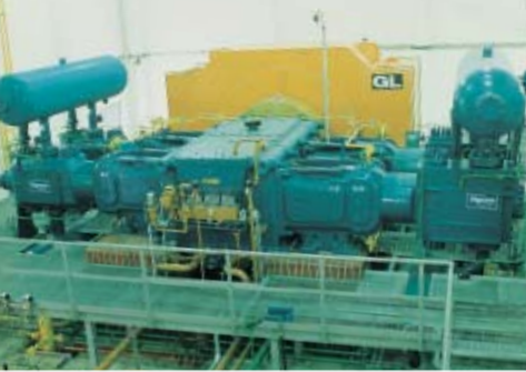
4HG compressor with variable speed electric motor.
