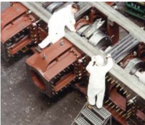
6HG crankcase with transverse spacers in place.
