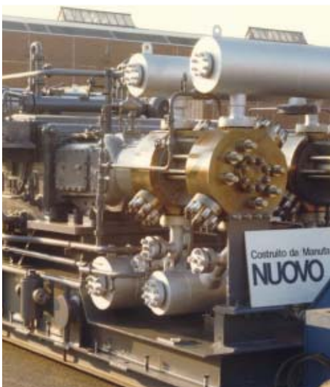
Re-injection compressor - model 4HE/2 at 370 bar.
