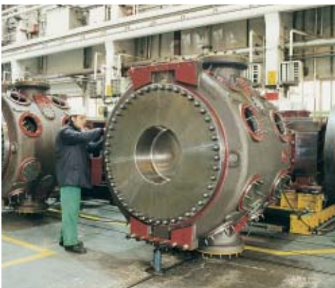
Large bore cylinder during assembly.
