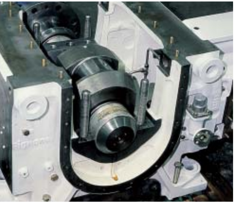
Main bearing split in the vertical plane.
