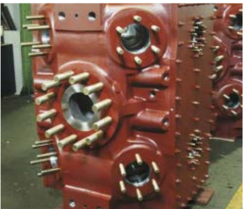
Cast steel cylinder before assembly of internals.
