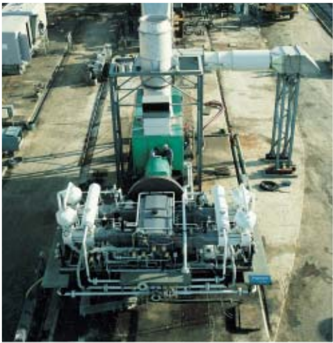
GE PGT5 gas turbine driven compressor during full load test.
