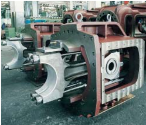
Crosshead extension before assembly on the crankcase.
