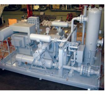
The VIP cylinder incorporates advanced technology that is matched by our proven frame. The 5B-VIP compressor has a 5" (127 mm) stroke and is rated up to 2125 hp (1585 kW) at a maximum 1500 rpm. The 6B-VIP compressor has a 6" (152.4 mm) stroke and is rated up to 1700 hp (1268 kW) at 1200 rpm.
