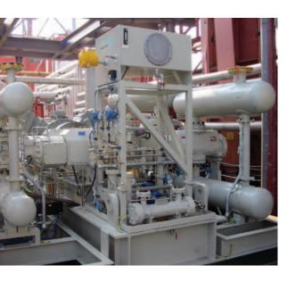
Dresser-Rand's VIP cylinder incorporates advanced technology that is matched by our proven frame. The 4C-VIP has a 4" (101.6 mm) stroke and is rated up to 2880 hp (2148 kW) at a maximum 1800 rpm. The 5C-VIP has a 5" (127 mm) stroke and is rated up to 2400 hp (1790 kW) at 1500 rpm. The 6C-VIP has a 6" (152.4 mm) stroke and is rated up to 1920 hp (1432 kW) at 1200 rpm.
