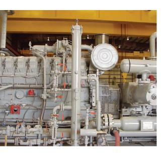
Dresser-Rand's D-VIP compressor uses unique design features of both the HOS and VIP compressors. Like the HOS compressor, the open-frametop construction of the D-VIP compressor ensures rigidity while providing large access areas for maintenance and inspection. Also featured is the throughbolt distance piece design for improved load-carrying capability. The D-VIP compressor also has some unique unloading features that make it one of the most versatile compressors available today.
