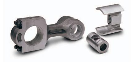
High-strength nodular iron crossheads feature shim-adjustable aluminum shoes at top and bottom. Crosshead pins are full-floating. Integral crosshead guide housings assure positive alignment with the frame.
