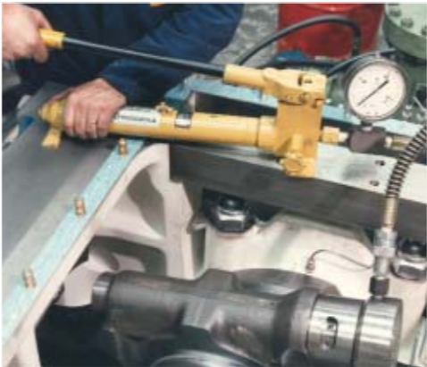
Connecting rod hydraulic tightening.
