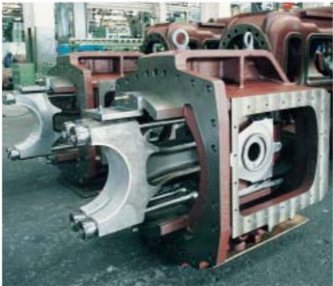
Crosshead extension before assembly on the crankcase.
