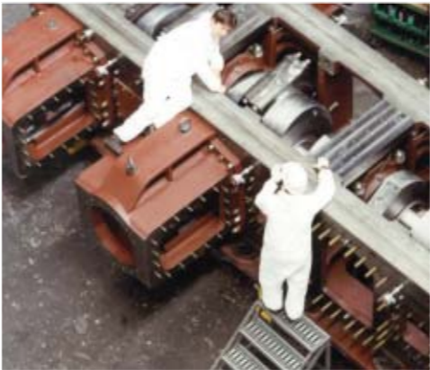
6HG crankcase with transverse spacers in place.
