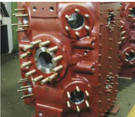
Cast steel cylinder before assembly of internals.
