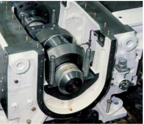
Main bearing split in the vertical plane.
