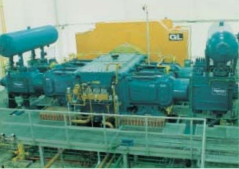
4HG compressor with variable speed electric motor.
