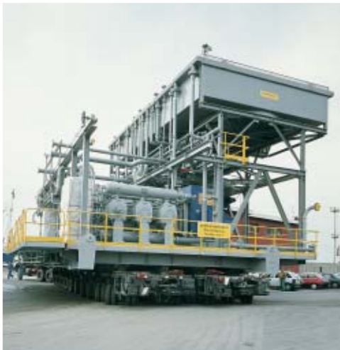
6HM reciprocating compressor offshore module during transportation.
