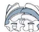
Fig 2 As the rotors mesh, the gas is trapped between the rotors and the casing.
