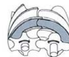
Fig 3 Continued rotation progressively reduces the space occupied by the gas, causing compression.
