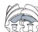
Fig 4 Compression continues until the interlobe space becomes exposed to the outlet port, through which the gas is discharged.
