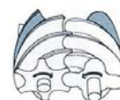
Fig 1 Gas is drawn in to fill the interlobe space between adjacent lobes.
